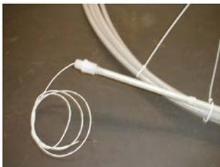
1. Using a side cutter, cut the tie wrap at the end of the probe.
