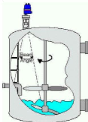
The two basic modes of operation are the “delta level” and “delta distance.” In the delta level mode, the current output (4-20 mA dc) increases as the liquid level rises. In the delta distance mode, the current output increases as the level falls (distance to the transducer increases). The desired span range may be set from a minimum of 3 inches up to 30 feet.
